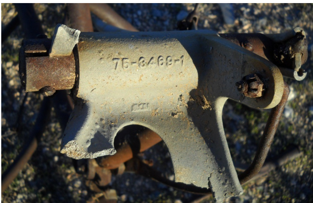
Rudder pedal with part number
