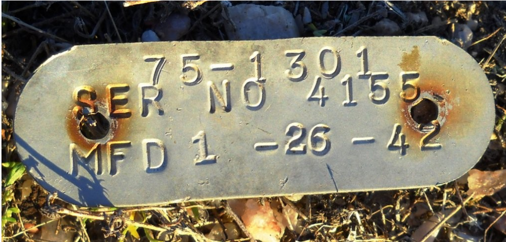
Tag with date of manufacture, serial number and part number that corresponds to the Frame Assembly, Center Section according to the parts manual. The aircraft was manufactured on January 26, 1942.
