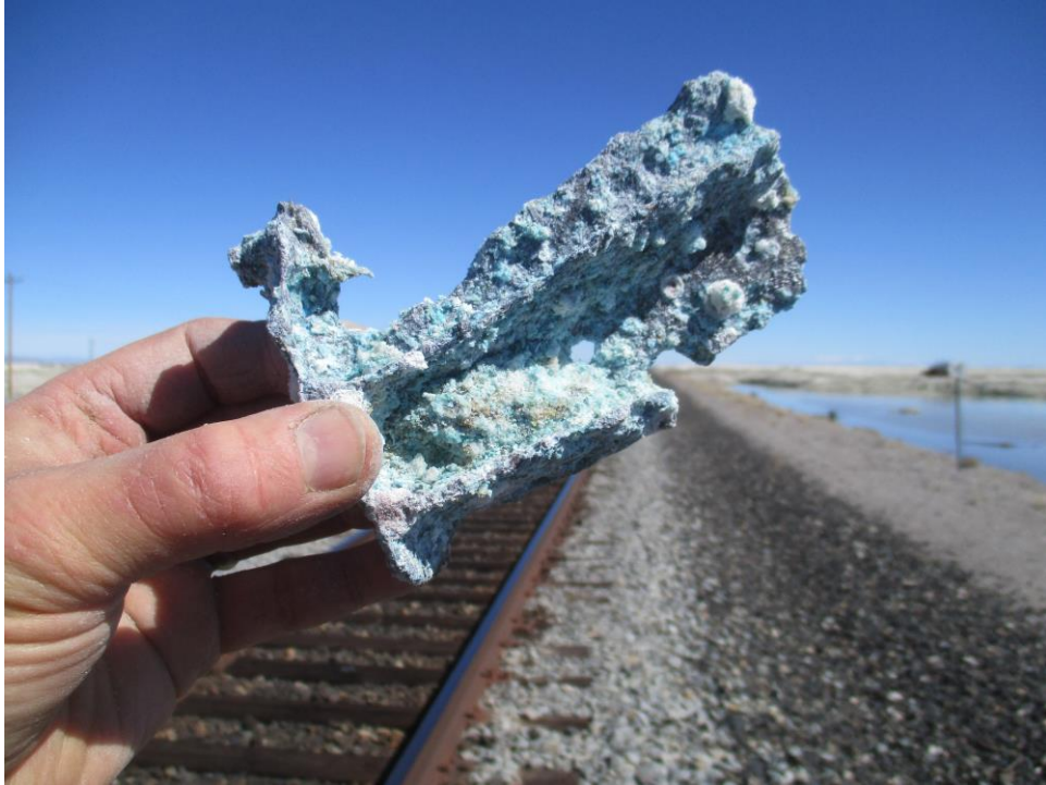
This oxidized structural piece turned blue after being buried in salt for nearly 80 years
