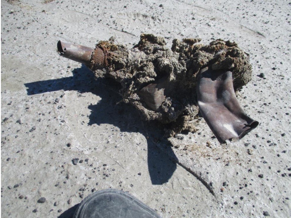
Part of a cylinder head from a Pratt & Whitney R-1830 engine
