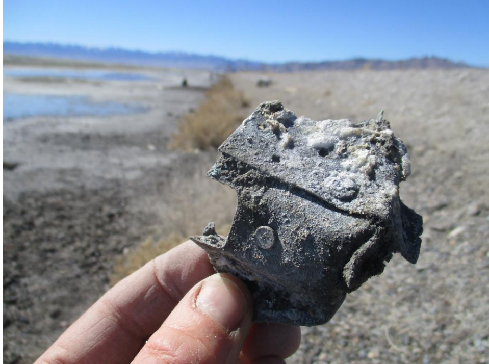
A couple of aircraft rivets are visible on this small piece
