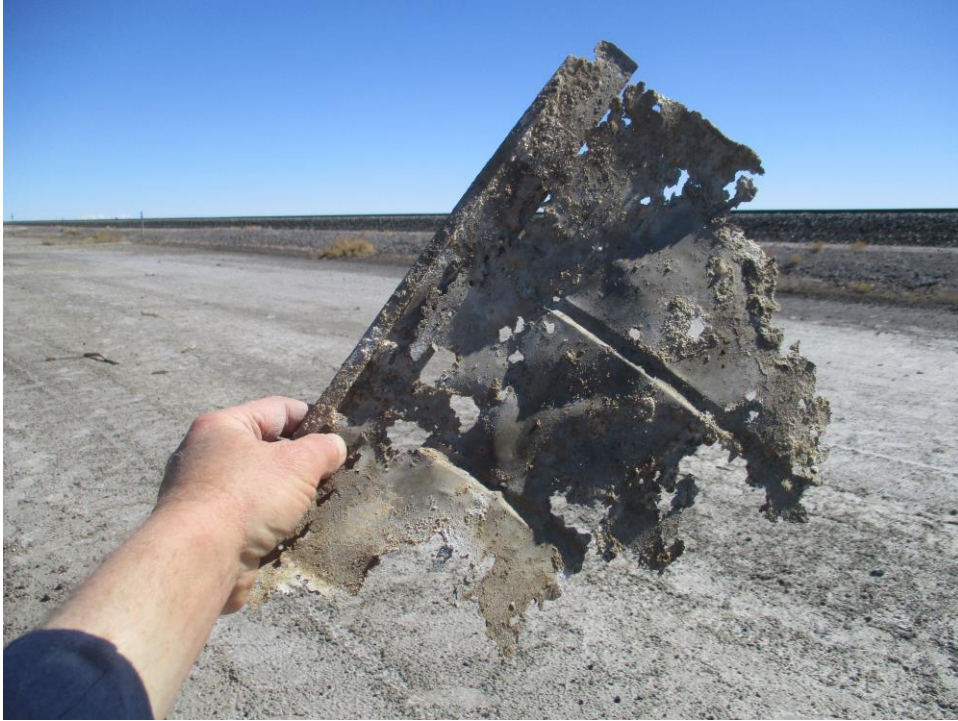
This aluminum piece shows how the salty soil in the area has damaged metal parts
