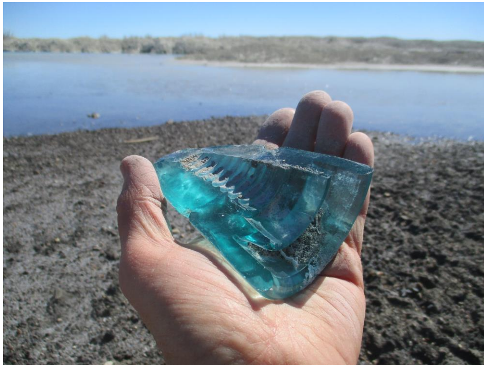
A broken glass insulator from the power lines
