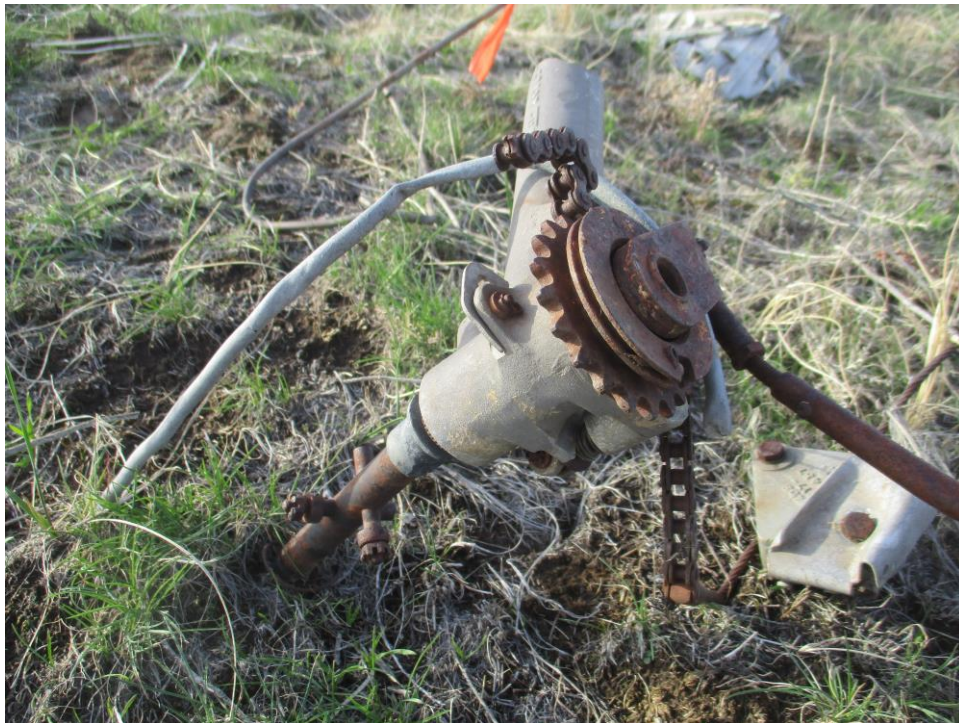
Chain and sprocket assembly for the flight controls
