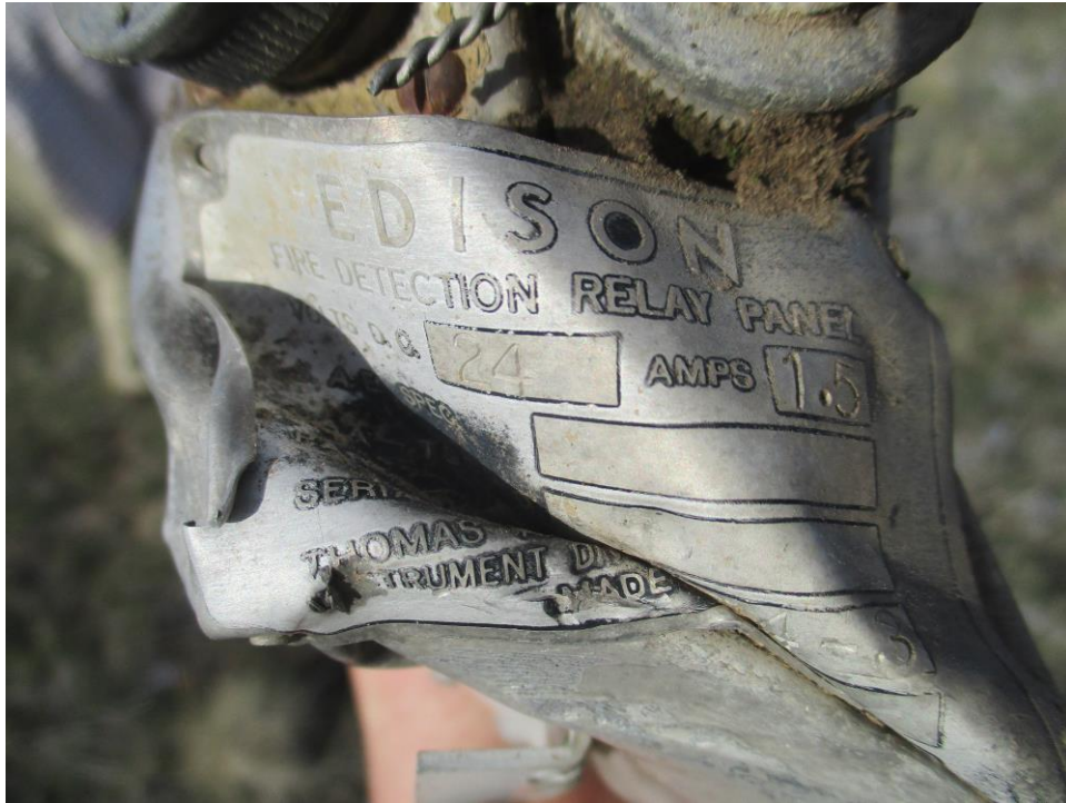
Data plate from the fire detection part
