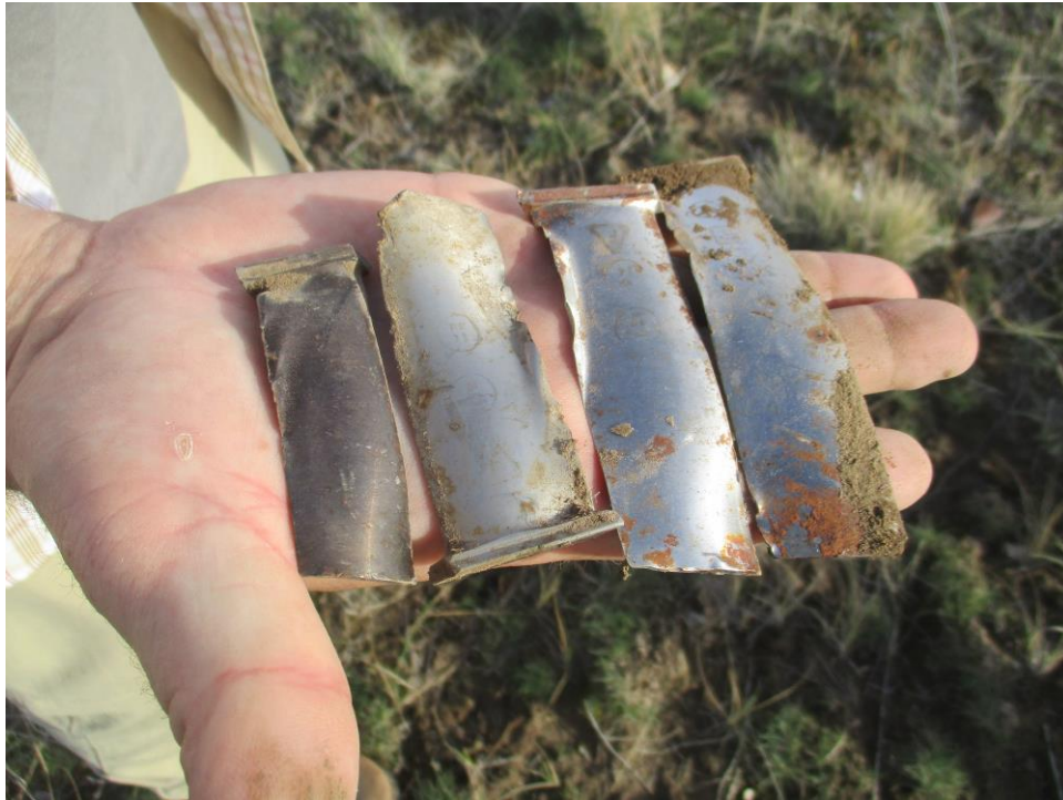
Compressor blades from the General Electric J47 turbojet engine
