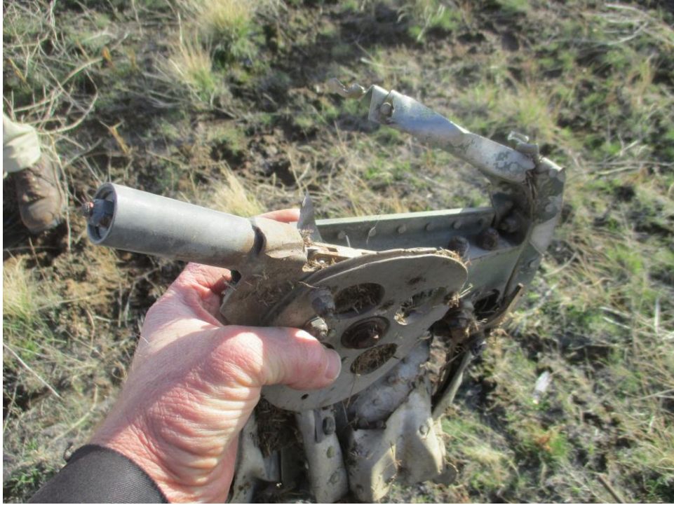
This piece had a grooved pulley for a control cable
