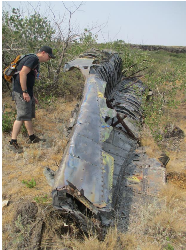
Aircraft mechanic Tate Ogden inspects the empennage of #65-0889
