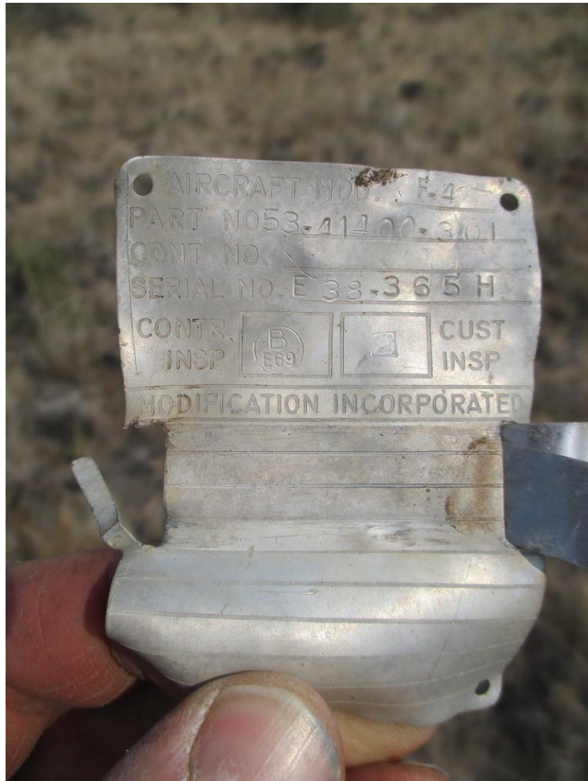
A data plate with the aircraft type stamped at top right
