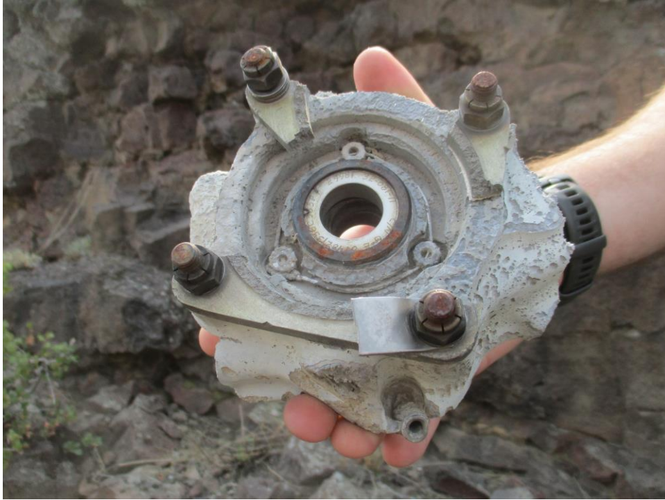
Part of a hydraulic pump
