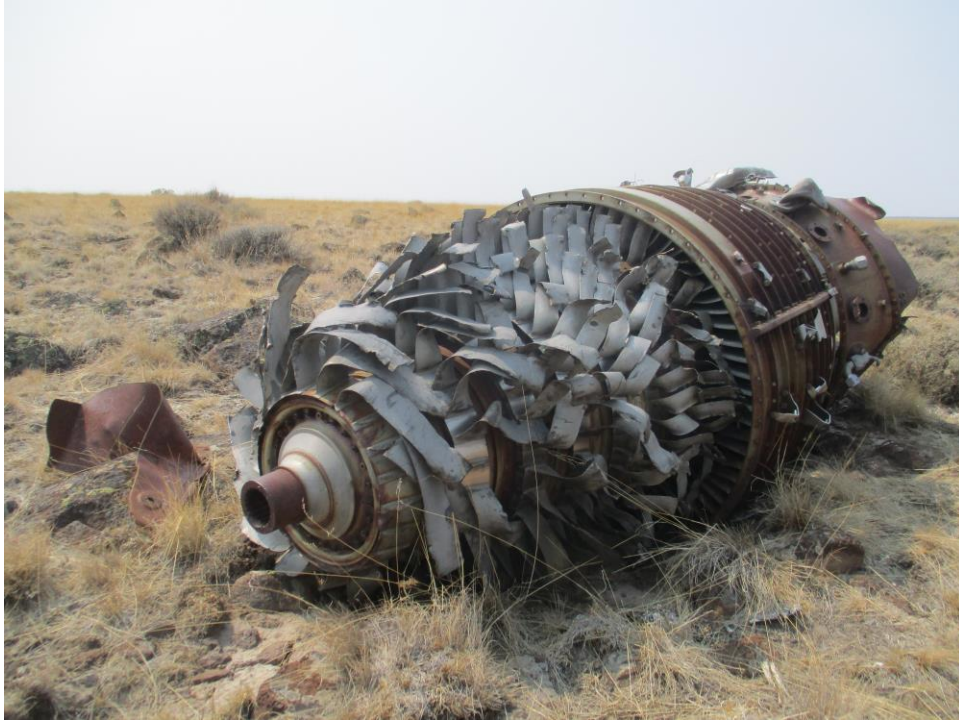
Another engine view. The rear half of each J79 has been removed by salvagers.
