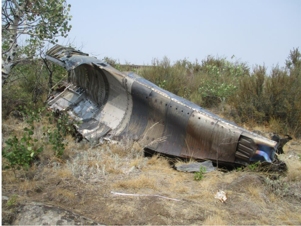
Another view of the empennage, which is missing the vertical and horizontal stabilizers
