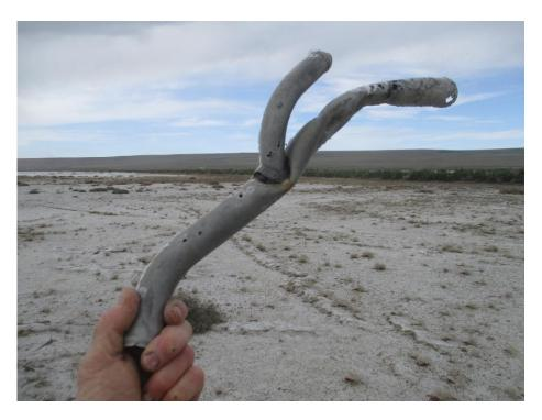
The holes in this aluminum tubing show how corrosive the salty soil is
