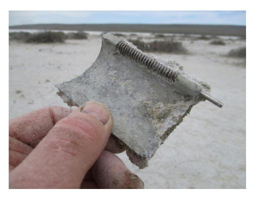
This curved piece has a spring-loaded hinge on it
