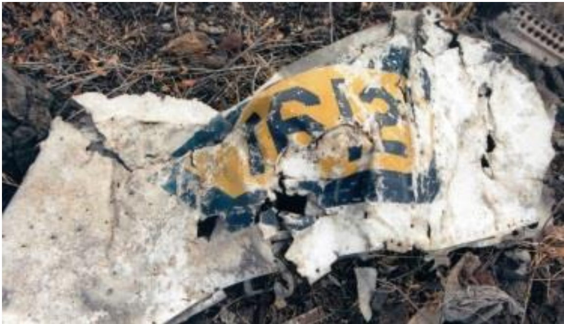
Nose gear door with last 4 digits of the BuNo recovered from the crash site
