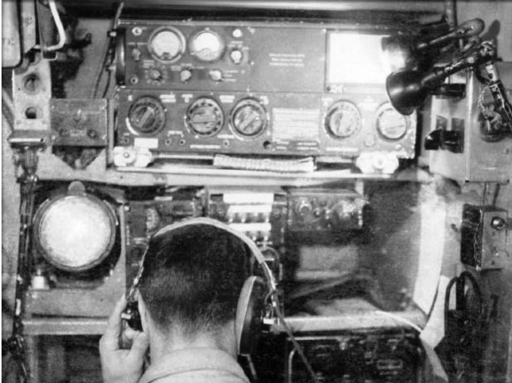
C-118 Liftmaster radio operator station with ART-13 Transmitter top center
