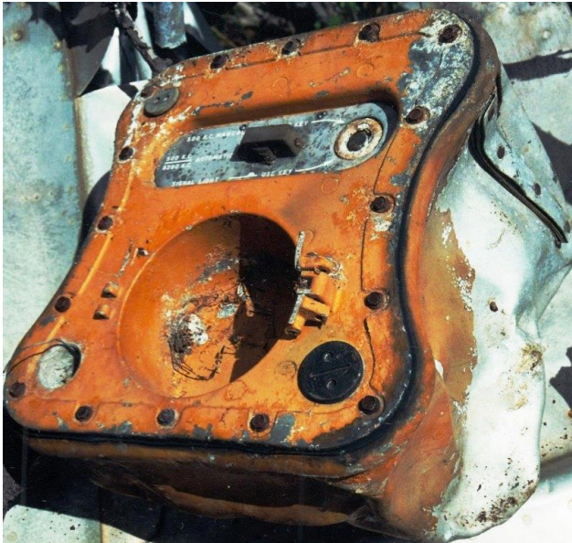
Two views of the wrecked BC-778 "Gibson Girl" emergency radio transmitter photos courtesy Don Hinton
