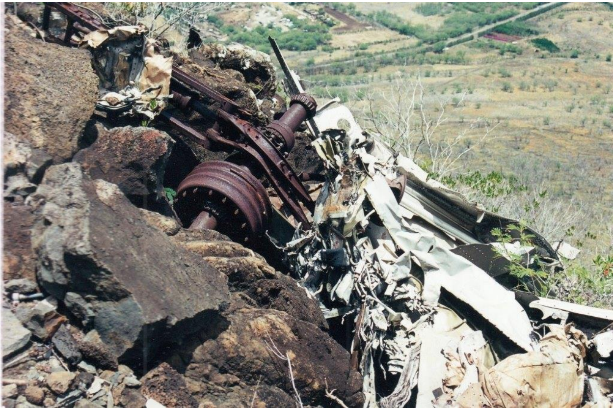
Main Landing Gear wreckage on steep slope photo courtesy Don Hinton
