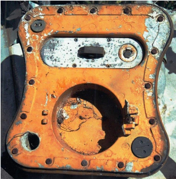
Two views of the wrecked BC-778 "Gibson Girl" emergency radio transmitter photos courtesy Don Hinton
